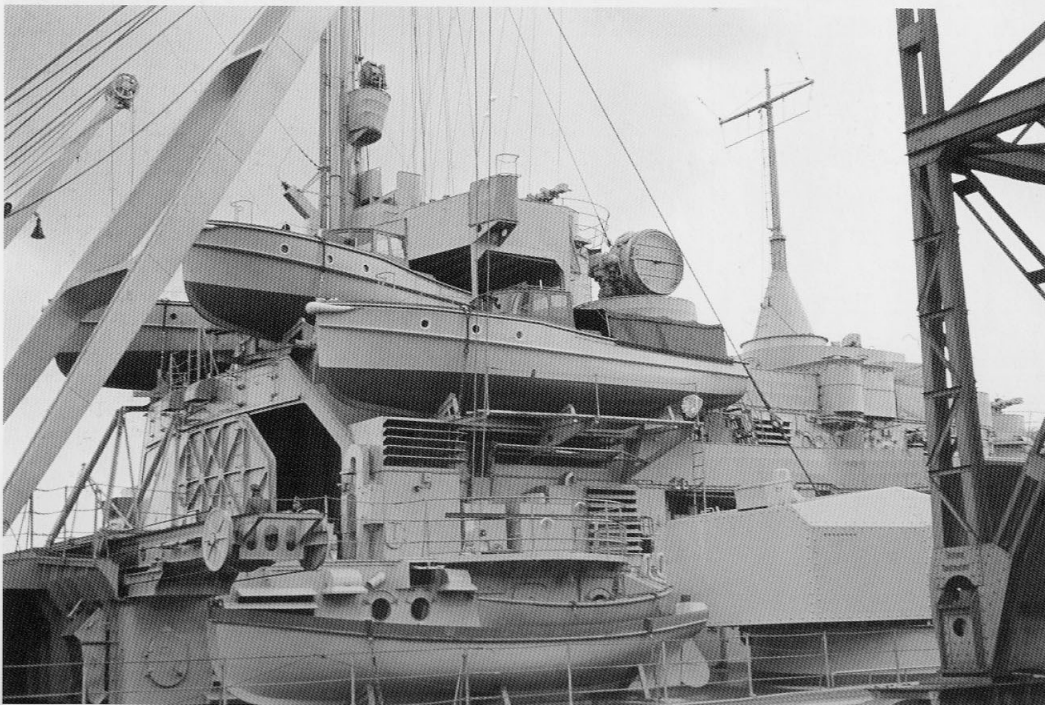
Bismarck August/September 1940: Portside view looking aft on Lower Mast Deck, showing 2cm gun (covered) and 4m SL8 rangefinder. (Ref. B193-18-6-25, Bundesarchiv)
