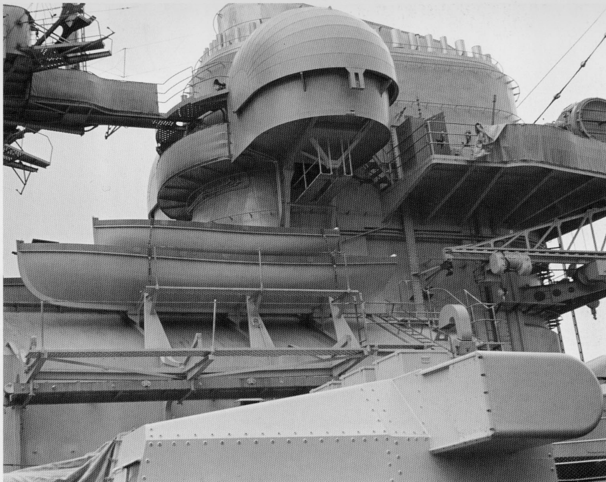
Bismarck August/September 1940: Portside view of the funnel and searchlight platform. The forward searchlight is covered. The port side Aircraft Hangar No. 2 can also be seen, with the 8m and 6m longboats lashed down on their stocks.
