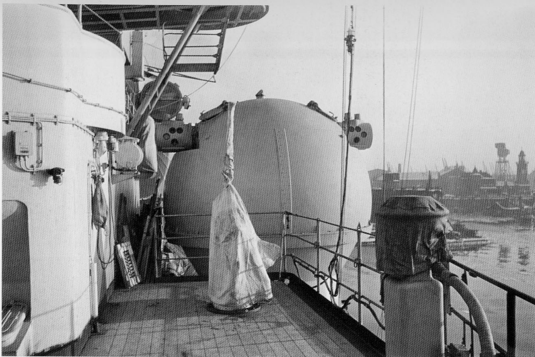
Bismarck August/September 1940: Portside view looking aft on Lower Mast Deck, showing 2cm gun (covered) and 4m SL8 rangefinder. (Ref. B193-18-6-25, Bundesarchiv)
